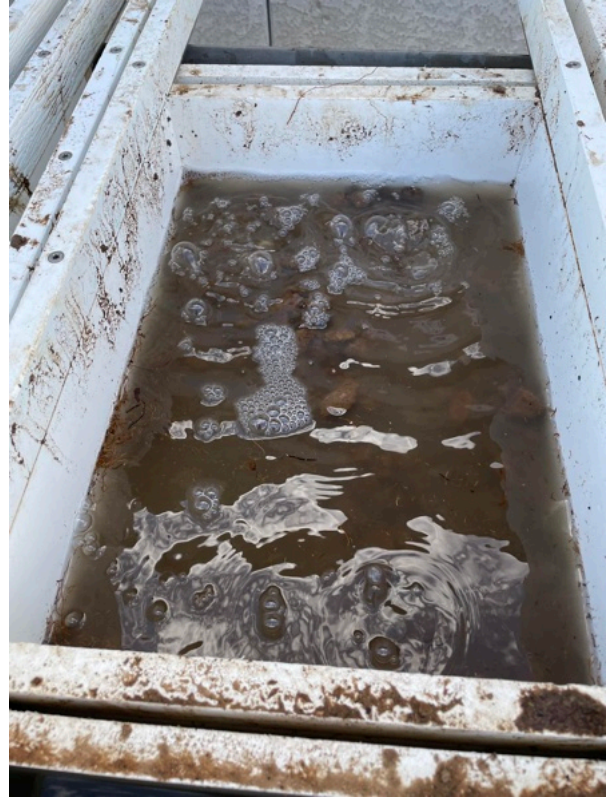
Above left and right. Collected sand and rock in giant trash bags is put into screens in a water-filled trough aka, "The Bubbler" that is attached to an air compressor. The concoction bubbles for about 12 hours, loosening the sand particles and microscopic fossils.
